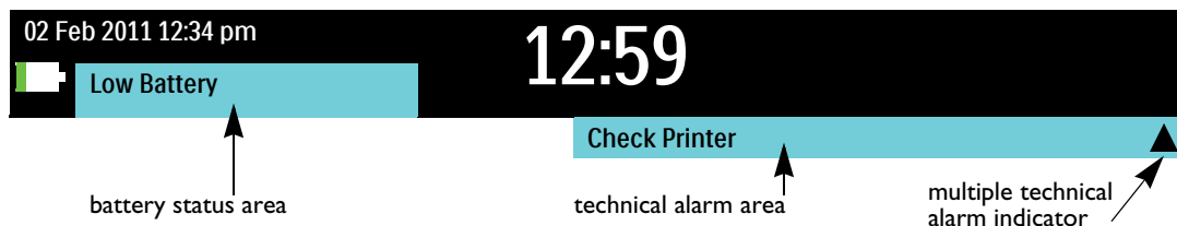
Figure 30 Technical Alarm Sample
